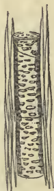
FIG. 66.—Thin section of Oakwood, magnified, showing a dotted vessel, between long wood-cells.
